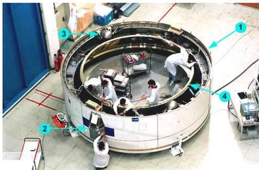
**Figure 3: Vehicle Equipment Bay containing System Control Attitude (SCA)**
