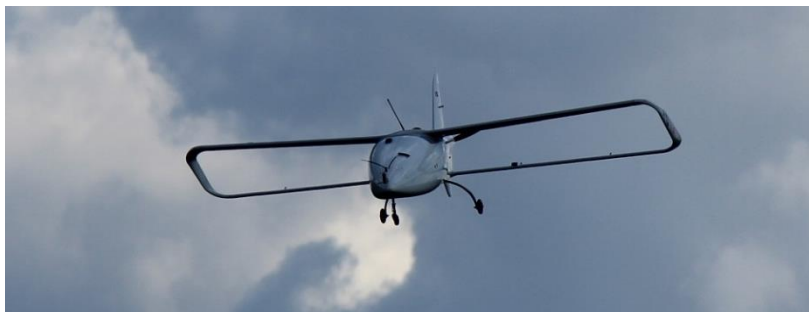
Fig. 1. MOSUPS aircraft on its maiden flight with unshrouded propeller
