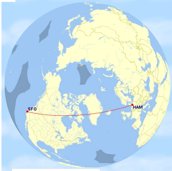
Figure 3: Example of ETOPS flight (Hamburg to San Francisco) with the Airbus A330 without an APU based on 120 minutes of ETOPS [16]
