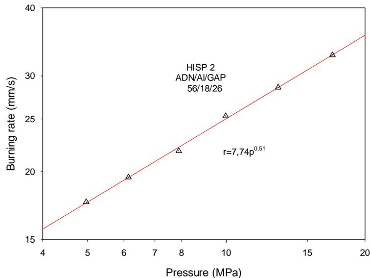
Figure 3. Burning rate for ADN/Al/GAP propellant, HISP 2.
