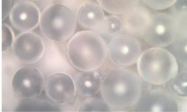
*Figure 1. Improved 100% dense ADN prills with reduced sensitivity.*
