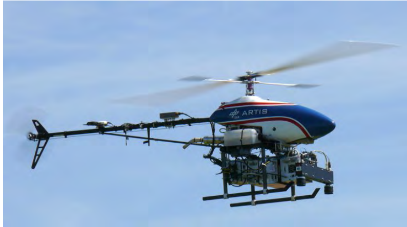
Fig. 1 DLR's 13 kg helicopter with a stereo camera, onboard image processing and GNSS/INS navigation filtering.
