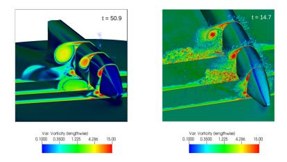
**Fig. 1** Instantaneous vorticity (in train length direction) for three different slices of the incompressible URANS (left) and DDES (right) simulation. Also shown is the stream-wise component of wall shear stress on the train surface. Time is expressed in units of convective timescales.
