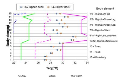
Fig. 4 Comparison of the equivalent temperatures for a passenger in the upper and lower deck.
