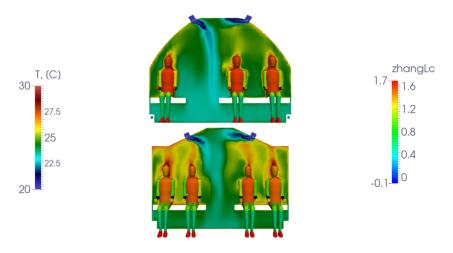
Fig. 3 Temperature distribution in a cross-section in the middle of the cabin and zhangLc indices on passenger bodies.
