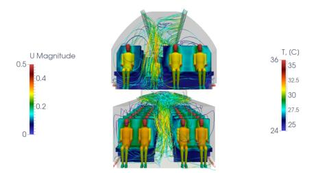
Fig. 2 Streamlines emerging from inlet surfaces colored with the velocity magnitude and temperature distribution on passenger bodies.
