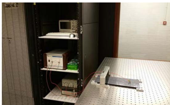
Figure 4 a) Ultrasonic verification setup with composite specimen mounted on the optical table. b) Schematic description of the ultrasonic verification equipment.
