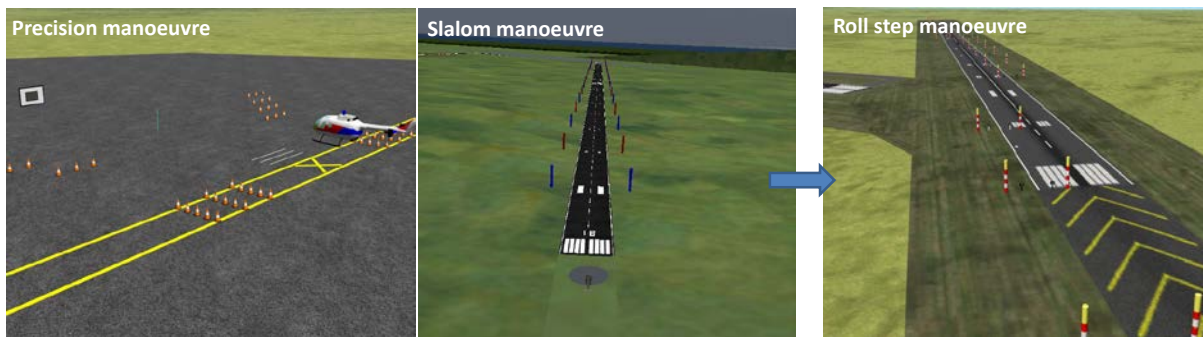
Figure 15 Manoeuvres flown to unmask RPC –University of Liverpool simulations [18]
