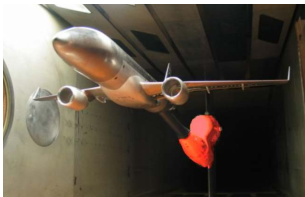
Figure 2: Example of model on rear sting with double roll boom
