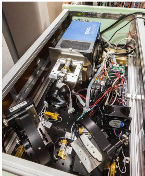
Figure 3: Pictures of a) camera module inside housing b) rear side of test section with camera housing in place, c) view through window frame from inside the test section.
