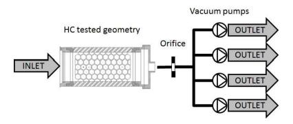
Figure 2: TEST RIG LAYOUT
