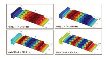
Figure 7: NUMERICAL EIGENMODES - GEO4
