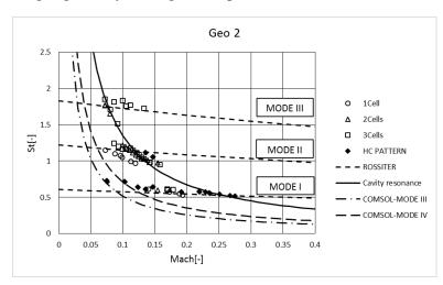
Figure 10: STROUHAL NUMBER FROM EXPERIMENT AND CORRELATION - GEO2 H/H0=2
