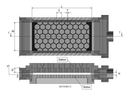
Figure 4: HONEYCOMB SEAL GEOMETRY
