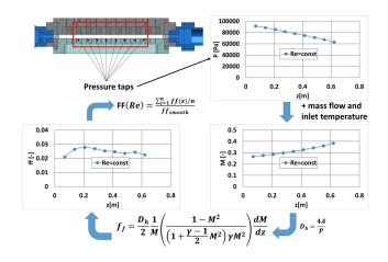
Figure 3: POST-PROCESSING FLOWCHART
