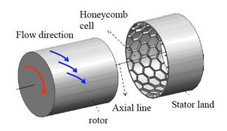
Figure 1: HONEYCOMB ANNULAR SEAL
