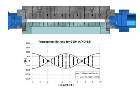
Figure 8: ACOUSTIC PRESSURE OSCILLATIONS
