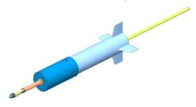
Fig. 5 sketch of harpoon for terrestrial demonstration, made up of conical tip to avoid debris generation and crushable cartridge to limit depth of penetration within debris.
