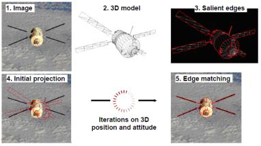
**Fig. 9**. Principle of tracking. Tracking is performed using a frame (1) and the 3D model of the target (2). The salient edges of the target are extracted (3) and projected into image (4), given an initial pose. Pose is iteratively refined to make projection edges match with image edges (5).
