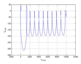
**Fig. 6**. Rendezvous performed using analytical guidance algorithm on quasi circular orbit (Prisma). The rendezvous duration is 64620 s (10 orbits) The error on the final state for this rendezvous is less than 1 cm in position, and around 1 mm/s in velocity.
