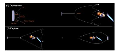
Fig. 4 . Deployment and capture sequence using a net
