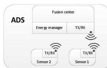
**Fig. 2** This scheme shows decentralized energy management for OWSAN. In this architecture, each node is equipped with a local energy manager which regulates the activities of that node.
