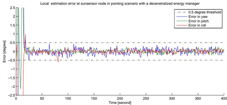
**Fig. 6** Simulation results of local attitude determination in sun sensor while decentralized energy manager scheme is operational.
