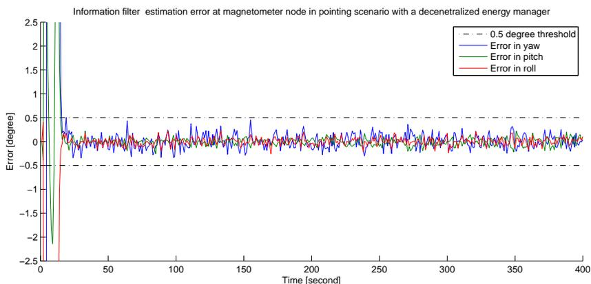
**Fig. 7** Simulation results of local attitude determination at magnetometer node while decentralized energy manager scheme is operational.
