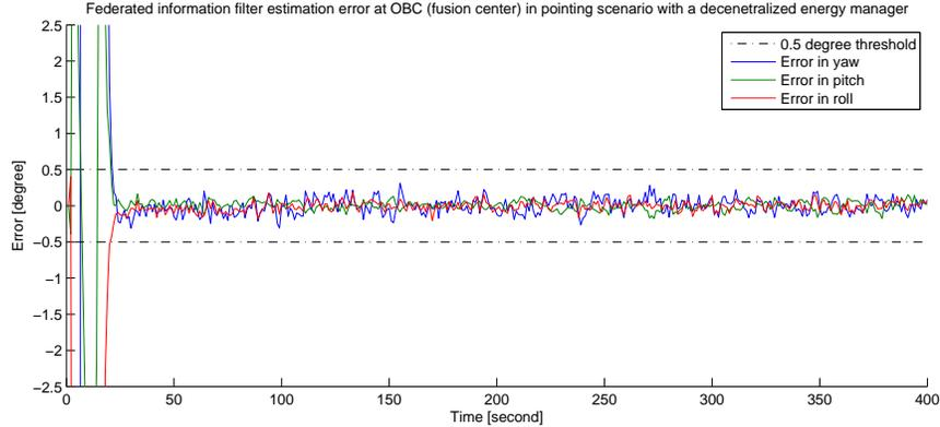
**Fig. 9** Simulation result of attitude determination at OBC. A federated information filter is used to produce attitude determination results at OBC for pointing scenario when decentralized energy management scheme is regulating the communication activity of sensor nodes.
