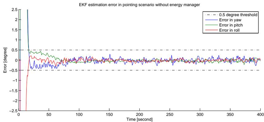
**Fig. 5** Simulation result showing the attitude estimation error in pointing scenario.
