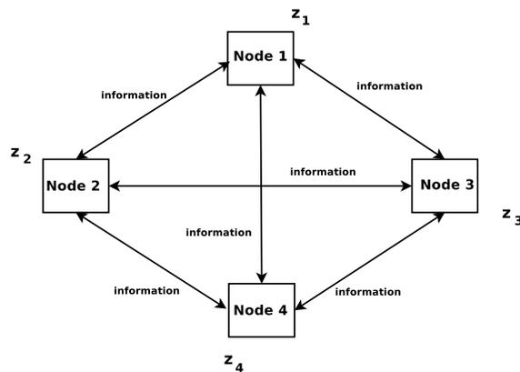
**Fig. 4** Decentralized scheme for OWSAN with two way communication channels and interconnected nodes.
