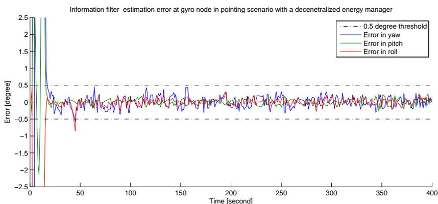
**Fig. 8** Simulation results of local attitude determination at gyro node while decentralized energy manager scheme is operational.
