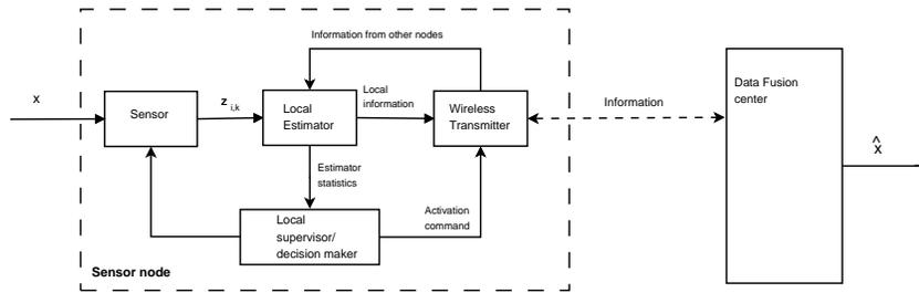
**Fig. 3** Structure of a sensor node in a decentralized architecture with local estimator and decision maker.
